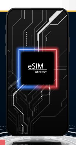
eSIMs (Embedded Subscriber Identity Modules) are digital SIMs that allow users to activate a telecom carrier's cellular plan without needing to obtain a physical SIM card. eSIMs are soldered directly to a board inside the user's device and (unlike traditional SIM cards) can store multiple operator profiles on a single module.
